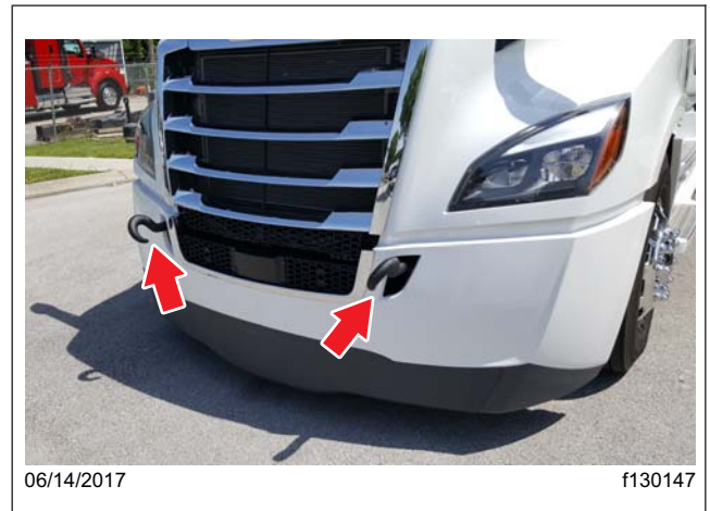
Fig. 2, Tow Hooks Installed, Facing Down
